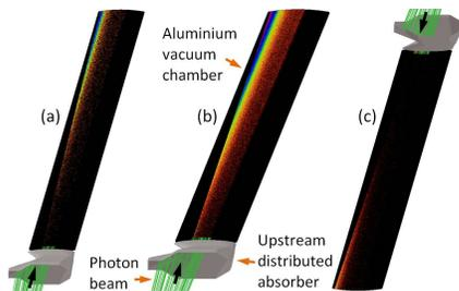
Footprint of the tails of BM radiation on the upper and lower walls of the aluminium vacuum chamber. (a) Nominal trajectory of the beam, (b) Radiation on the upper wall under vertical misalignment effect, and (c) Radiation on the lower wall under vertical misalignment effect.
