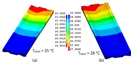
Thermal results for the aluminium vacuum chamber. The BM radiation is deposited on the upper and lower walls. (a) Temperature map for nominal trajectory of the beam. (b) Temperature map for trajectory of the beam under vertical misalignment effect
