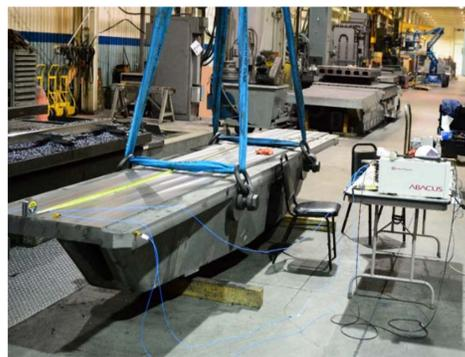
Figure 1: The FODO prototype girder casting at the manufacturer, rigged for a free BC EMA. Impact excitation, roving accelerometer.
