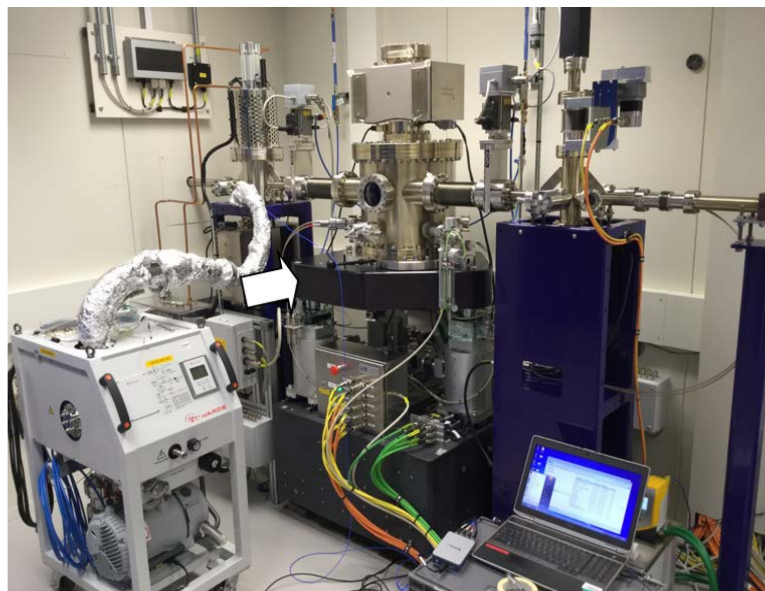
Figure 2: Mirror System I08-M4 at the Diamond Light Source. Modal Analysis Impact location & Direction indicated by arrow
