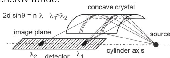
Principle of the von Hamos design, where a thin crystal is bent to a cylindrical surface [1,2].
