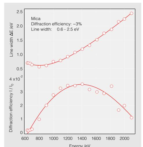
Diffraction from a thin mica crystal measured at the Optics beamline at BESSY/HZB.
