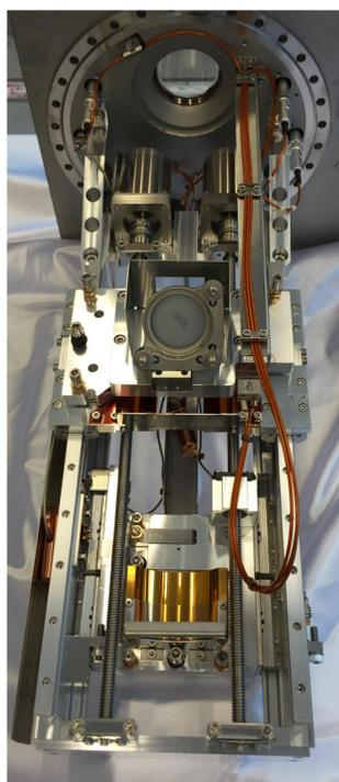
Internal mechanics of the von Hamos spectrometer.
