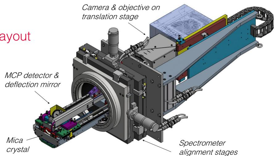
Using a high speed camera (500.000 frames/s at 1024x16 pixels) up to 400 spectra can be recorded within a macro bunch (10 Hz) of the European XFEL.
