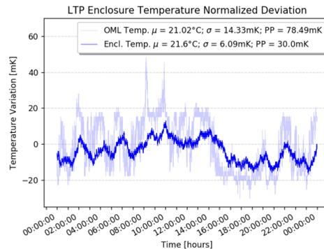
Figure 5: Normalized Temperature Variation at the OML room and inside the LTP enclosure
