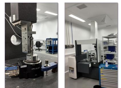
Spindle Error Analyzer (left) and Coordinates Measuring Machine (right)
