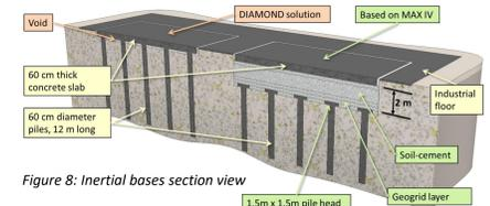
Figure 8: Inertial bases section view
