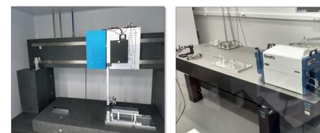
LTP (left) and Fizeau Interferometer (right) at the OML
