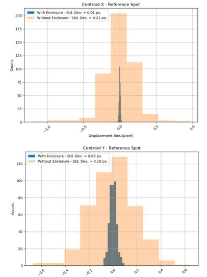
Figure 6: Comparison between position stability during a short period measurement of a reference mirror, inside and outside the LTP enclosure
