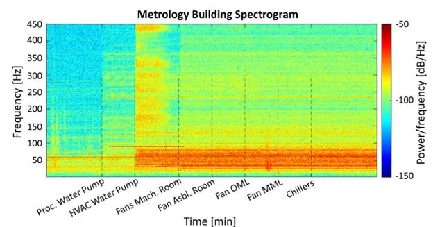
Figure 9: Frequency contribution analysis on HVAC machinery sequential start
