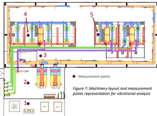
Figure 7: Machinery layout and measurement points representation for vibrational analysis
