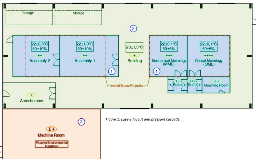
Figure 1: Layers layout and pressure cascade.
