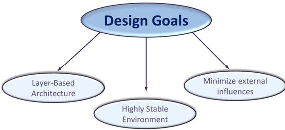
The LNLS Metrology Building was designed following a layer-based architecture: the outer layers have a proper environmental control that contributes for the stability of the inner ones. The goal is to provide the laboratories (inner layers) a highly stable environment, minimizing the influence of the large thermal and humidity variations that may occur outside the building
