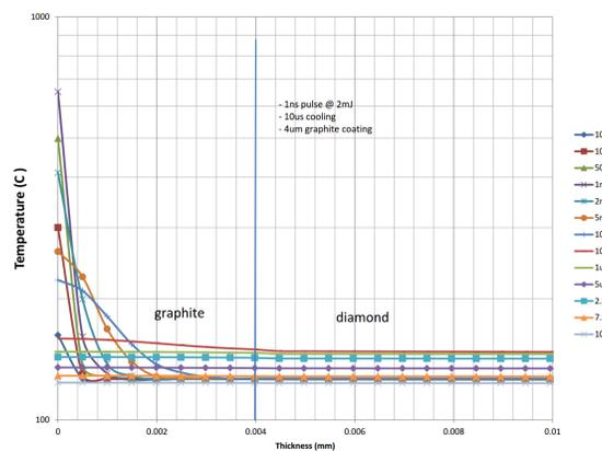
Single pulse transient thermal in graphite coating to diamond
