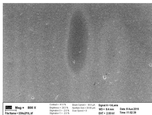
Damage test, 0.6eV/atom, graphite coated diamond
