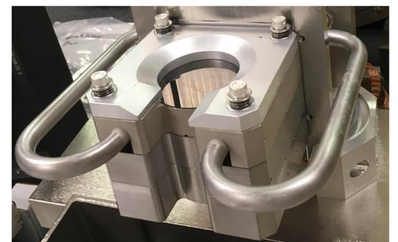
Absorber assembly with graphite coated diamond and light-tight box
