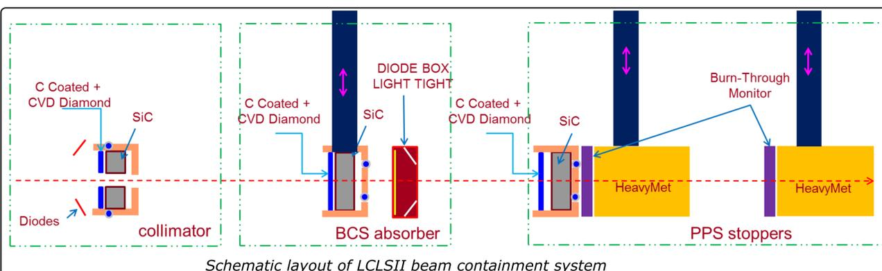
Schematic layout of LCLSII beam containment system
