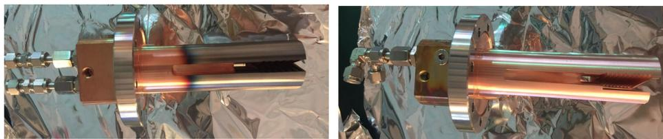
Figure 1: 1<sup>st</sup> absorber with NEG coating
