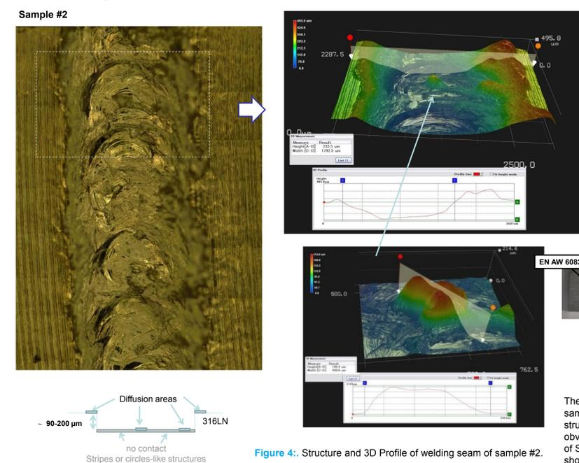
Figure 4: Structure and 3D Profile of welding seam of sample #2.
