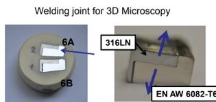
Welding joint for Hardness, X-Ray fluorescence, SEM/EDX & 3D Microscopy
