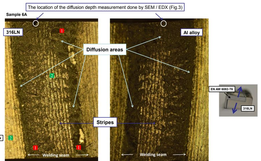
Figure 5: Structure of welding seam of sample 6A. Mirror display of two opposite surfaces of the welding joint of sample 6A. The green and red squares show the location of measurements of chemical composition by X-Ray fluorescence.
