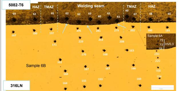
Figure 1: Distribution of HV1 hardness values measured along welding seam area and TMAZ/HAZ areas of sample 6A/6B. Arrows show the small particles of stainless steel fraction mixed by welding with Al alloy. Insert shows the hardness of sample 6A.
