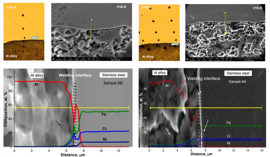
Figure 3: Concentrations profiles of Fe, Ni, Cr and Al across the EDX analysis line at the welding interface between Al alloy and stainless steel.
