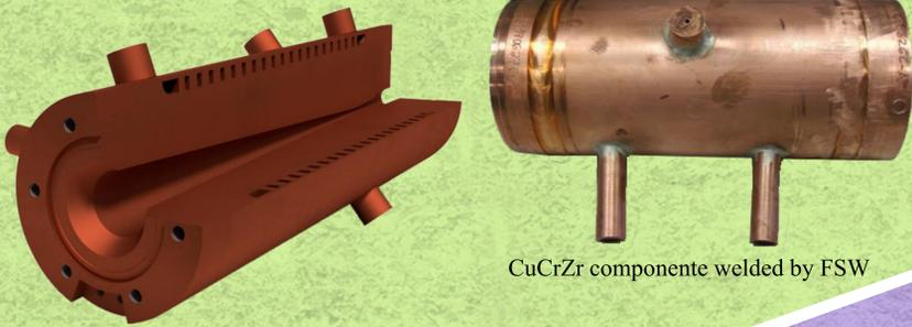
CuCrZr componente welded by FSW
