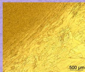
Microstructure of a FSW welded region.
