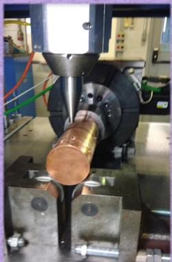
Friction Stir Welding (FSW) on a CuCrZr component.
