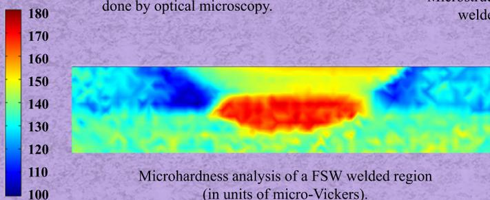
Microhardness analysis of a FSW welded region (in units of micro-Vickers).
