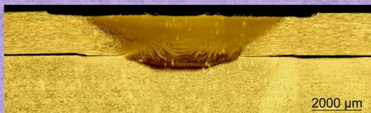
Cross-section image of the welded region done by optical microscopy.
