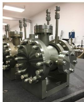
Photon Collimator vacuum chamber assembled
