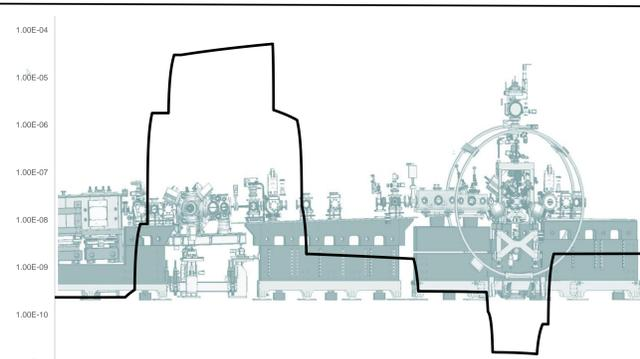
The large range of vacuum pressure used in the 2 main end stations requires sophisticated pumping options and numerous differential pumping systems between the essential elements of the beam-line. The LAMP end station will work at levels of up to 10<sup>-5</sup> torr, while the DREAM end station will continuously work in the low 10<sup>-11</sup> torr range.
