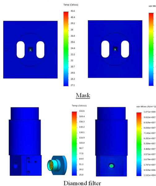
Figure 5: The result of thermal simulation representing the temperature and thermal stress for the mask and diamond filter.
