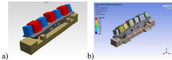
Figure 4: Grouted FODO prototype, first mode shape comparison, a) is EMA at 41 Hz, while b) is FE modal analysis at 42 Hz (2.4% difference).
