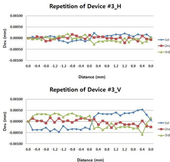
Figure 4: Repetition of cavity BPM Mover. Maximum deviation is ±0.3 μm of horizontal and ±0.6 μm of vertical measurement for number 3 Mover.
