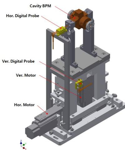
Figure 2: 3D view of cavity BPM Mover.
