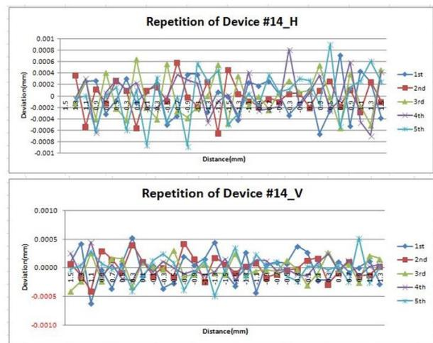
Figure 6: Repetition of Quad Mover. Maximum deviation is ±0.8 μm of horizontal measurement and vertical is ±0.6 μm for number 14 Mover.
