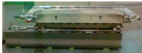
Figure 2: New Hall probe bench based in step motors.
