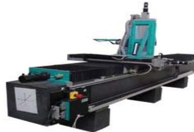
Figure 1: Old Hall probe bench based in DC motors upgraded in 2016.
