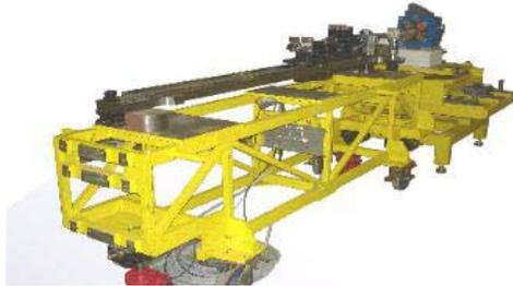
Figure 6: Old rotating coil bench.
