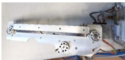
Figure 1: Existing ISOLDE beam needle scanner.
