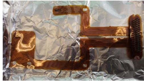
Figure 6: ISOLDE SEM grid FLEX cable.
