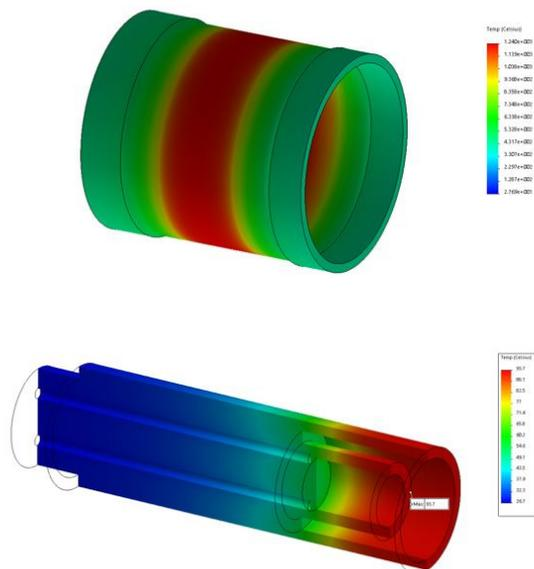
Figure 9: Filter cup and fixed jacket maximum temperature of 1240 °C and 94 °C respectively.
