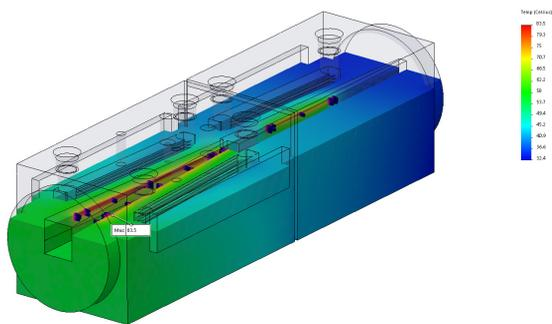
Figure 7: Shutter maximum temperature distribution.
