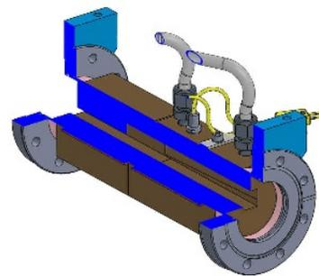
Figure 6: Photon shutter sectional view.
