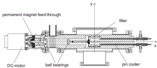
Figure 8: sectional view of rotating filter.
