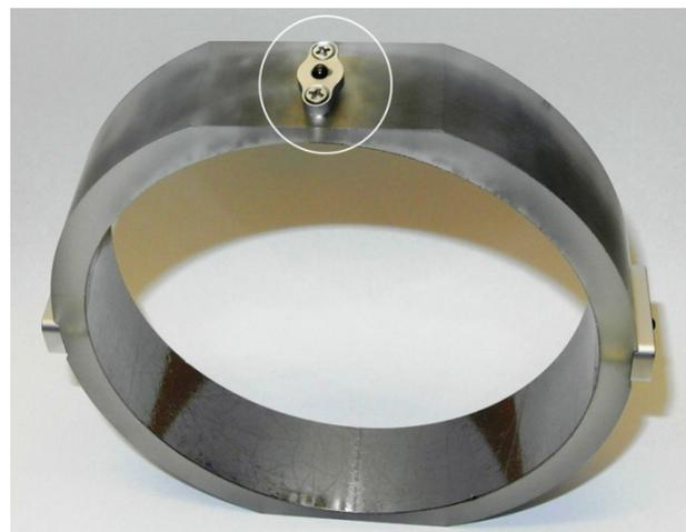
Figure 4: HAPG optics with three ball joints.
