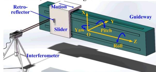
Figure 1: The diagram of angle deviations of the guideway.
