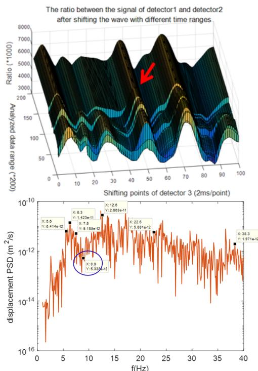
Figure 7: Vertical PSD spectrum of ground motion measured by five seismometers placed in 2#, 3#, 4#, 6#, 8# holes.
