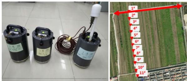
Figure 6: The seismometers used for the ground motion measurement of HEPS (left) and the measurement position on HEPS site (right).
