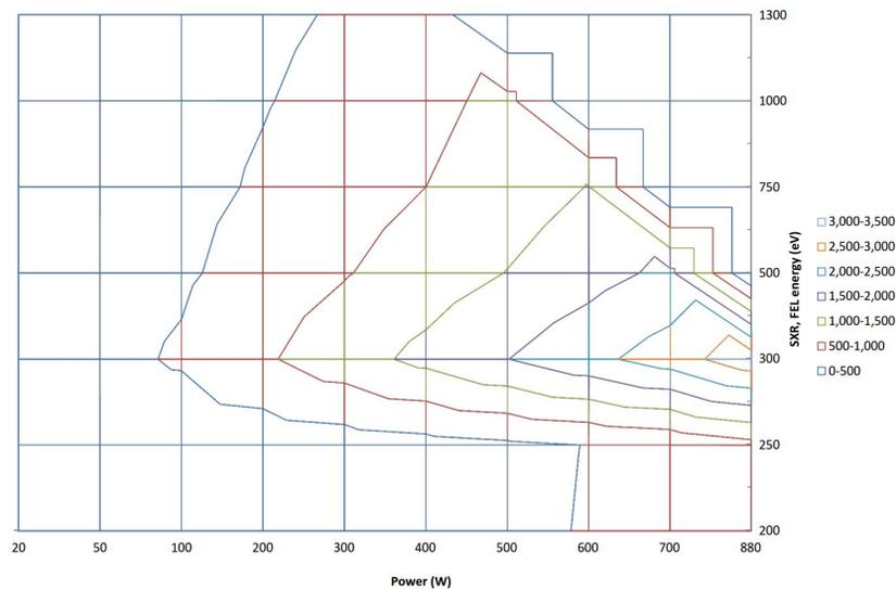
Figure 5: Temperature map on photon energy and power.
