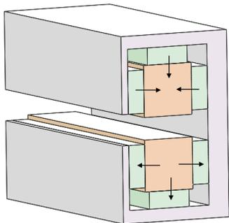
Figure 1: One module of the PM dipole.
