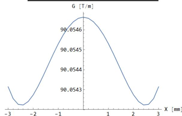
Figure 8: Homogeneity of quadrupole field.
