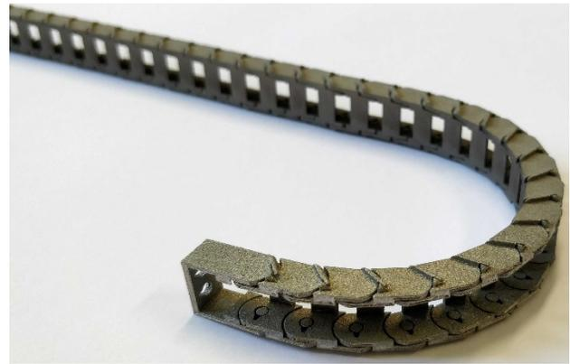
Figure 5: Titanium cable chain made by SLM.
