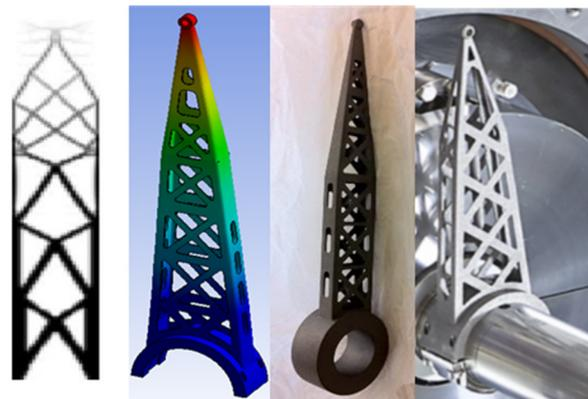
Figure 3(a-d): Design and production process for titanium wire scanner forks, showing successively: Optimisation; analysis; SLM product and finished fork.
