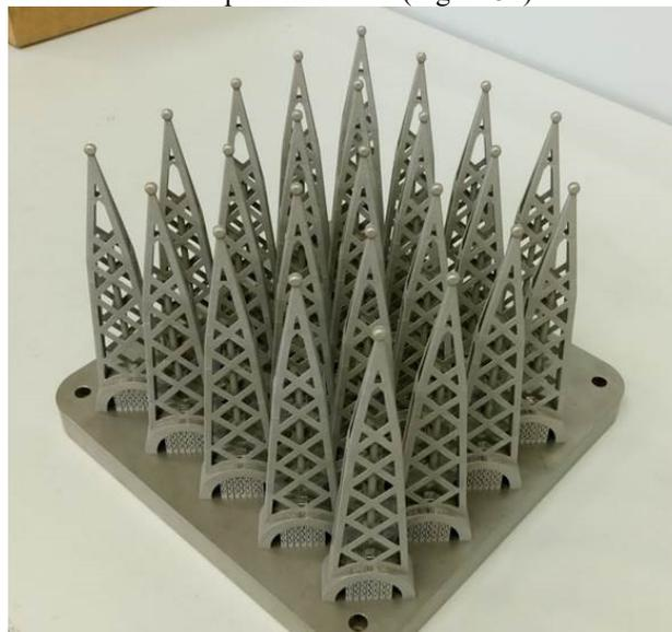
Figure 4: Series production of wire scanner forks.
