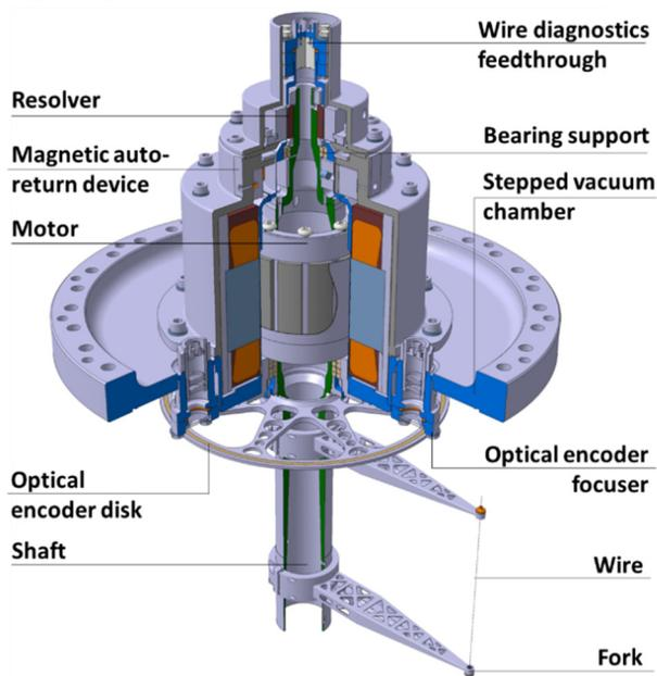
Figure 2: Part-section of the new wire scanner design showing the fork and wire.
