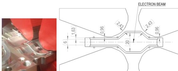
Figure 3: Picture and drawing showing the limited space available between the chamber and the pole tips. Heating wire elements are visible.
