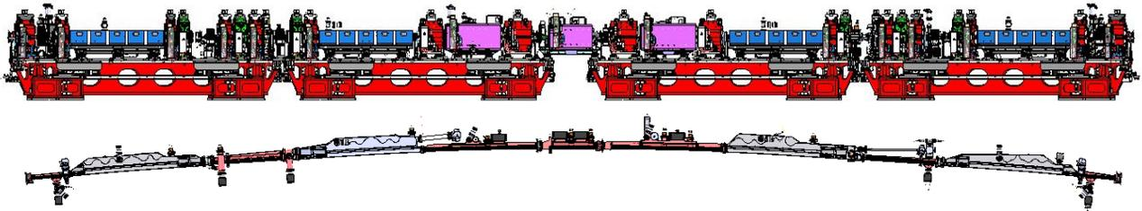
Figure 1: Front view of a cell (upper figure) and top view of the corresponding vacuum assembly (lower figure). Stainless steel chambers are highlighted in red in the lower figure.
