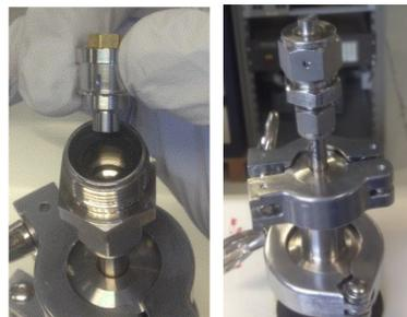
Figure 6: Leak detection device for an individual BPM button.
