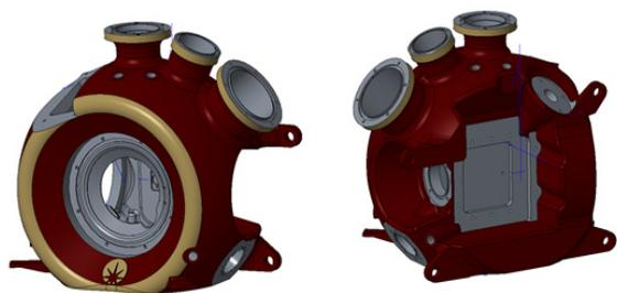
Figure 5: VMXm sample vessel designed for DMLS.
