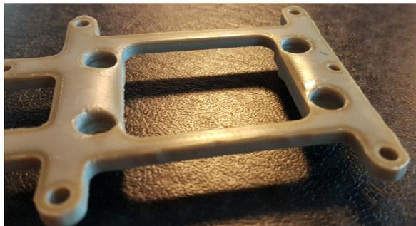
Figure 2: Component D, shown with base plate build surface facing upwards. Clear warping can be seen in the reflections.
