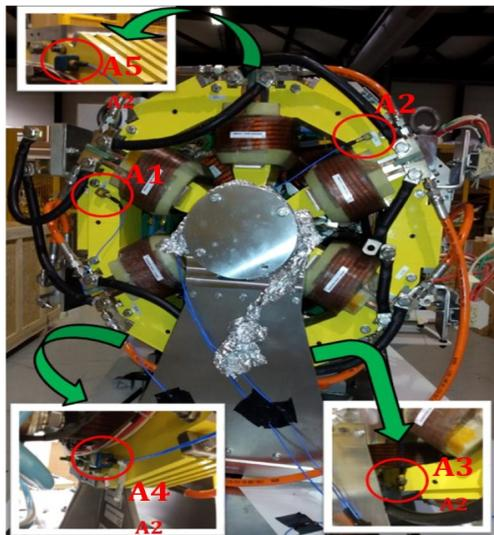
Figure 2: Positions of the accelerometers for the Sextupole.
