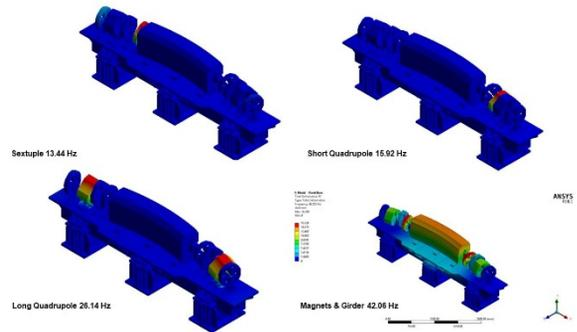
Figure 6: Girder & Magnets Assembly Mode Shapes.
