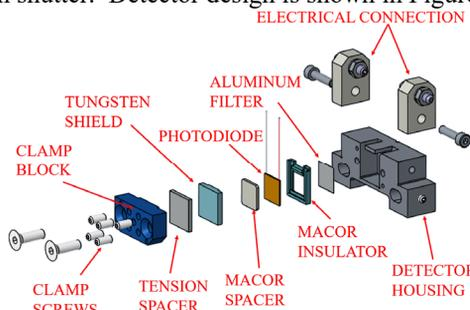
Figure 6: Detector Assembly for the IM1.
