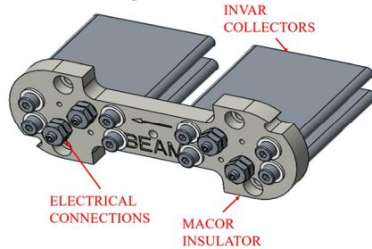
Figure 8: Photoelectron Collector for XBPM2.
