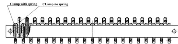
Figure 4: Final assembly of wire tighten component.
