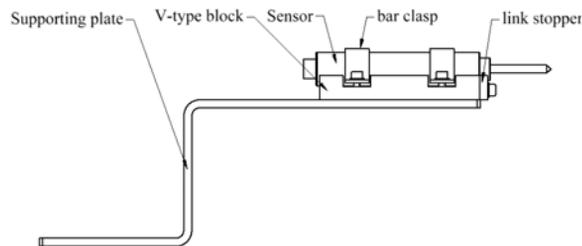
Figure 8: Located mechanism of displacement sensor.
