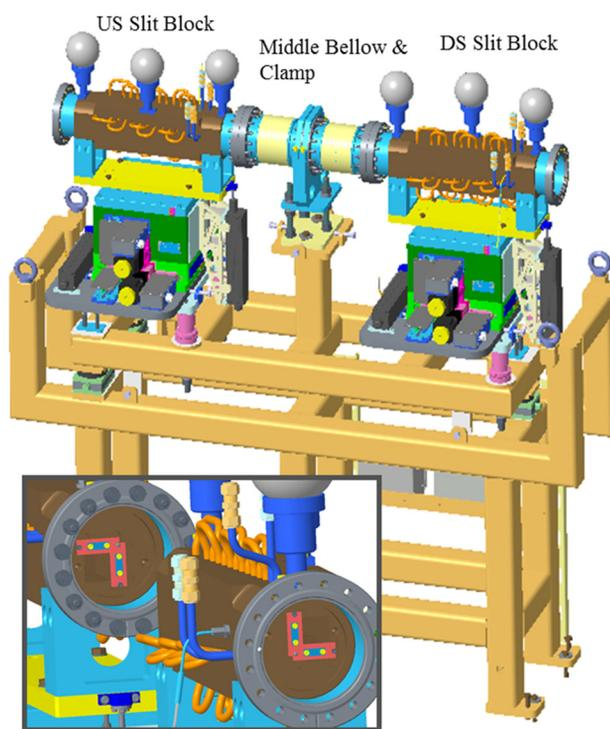
Figure 4: the DIAD front end slits. The detailed view shows the arrangement of the L shaped slit blades. The fabrication design from FMB Berlin [4] is shown here.
