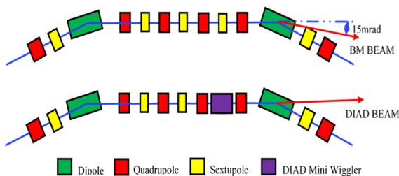
Figure 1: Top: Schematic diagram of the double-bend achromat layout. Bottom: Schematic diagram of the mini-wiggler replacing the sextupole.
