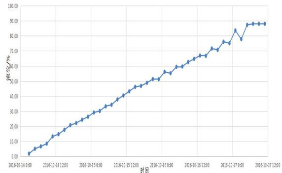
Figure 6: Liquid He accumulation curve of the SCU prototype.
