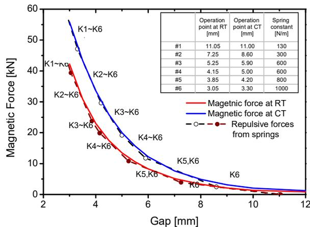
Figure 4: Dependence of magnetic (solid lines) and repulsive (dashed lines) forces on gap size at 300 K and 77 K.
