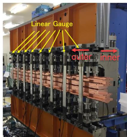
Figure 5: Gap error measurement setup on out-of-vacuum girder.
