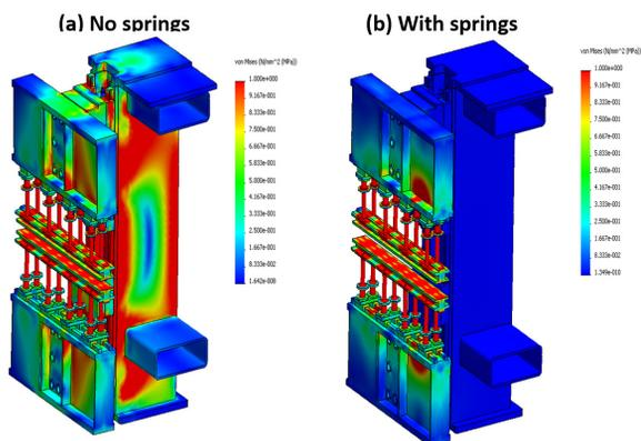
Figure 2: Stress distributions of the mechanical CU15 frame with and without spring modules under magnetic load of 32 kN.
