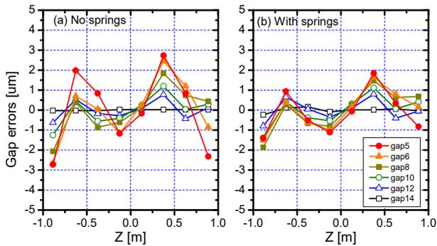
Figure 6: Effect of spring modules on gap errors for out-of-vacuum girders.
