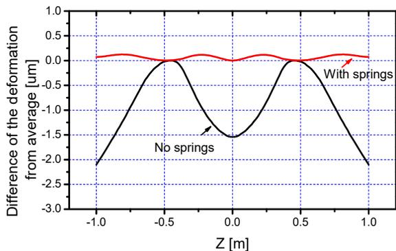
Figure 3: Finite element analysis on a deformed out-of-vacuum girder with and without spring modules under magnetic load of 32 kN.
