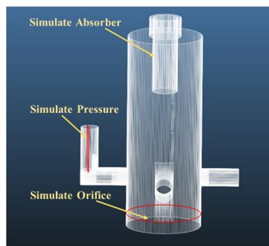
Figure 3: Simulation model.
