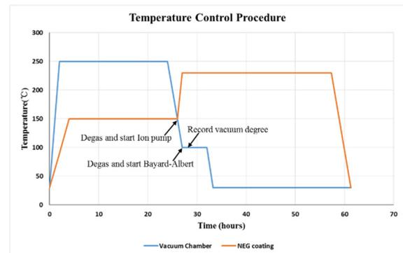
Figure 4: Temperature Control Procedure.
