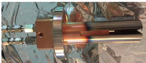
Figure 1: 1<sup>st</sup> absorber with NEG coating.
