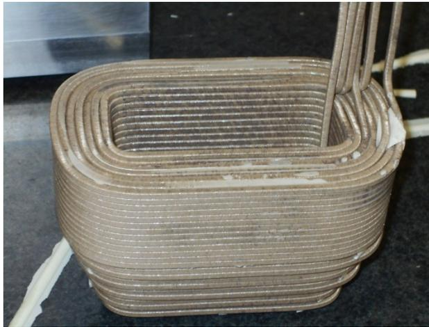
Figure 3: Prototype Wound Coil.
