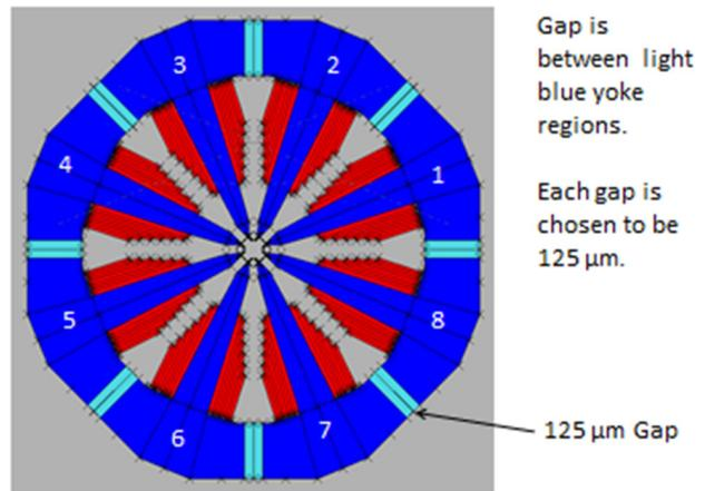
Figure 8: 2-D Model for the Pole Segment Gap Study.
