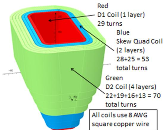
Figure 2: Coil Configuration.
