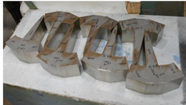
Figure 5: Prototype Bonded Pole Segments.
