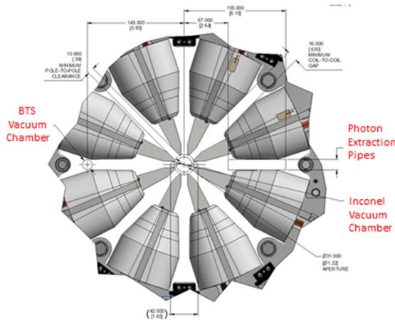
Figure 7: Vacuum System Component Clearance.
