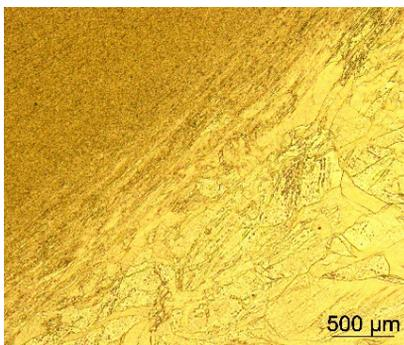
Figure 3: Microstructure of a FSW welded region.
