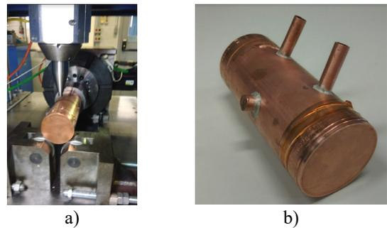
Figure 1: (a) Friction Stir Welding (FSW) on the CuCrZr component. (b) FSW-welded component.
