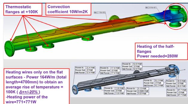
Figure 5: Thermal calculations
