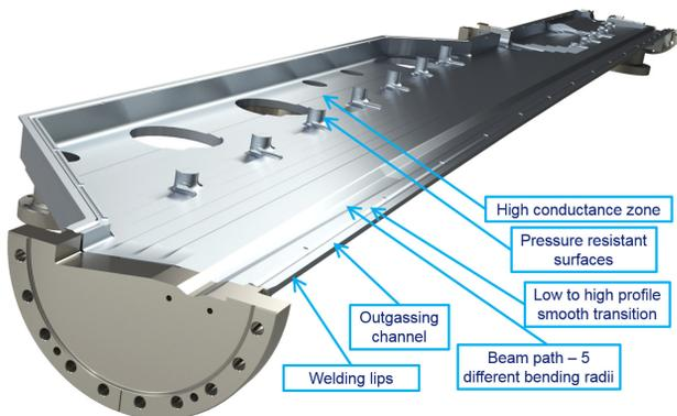
Figure 3: Bodies and welding (CH9).
