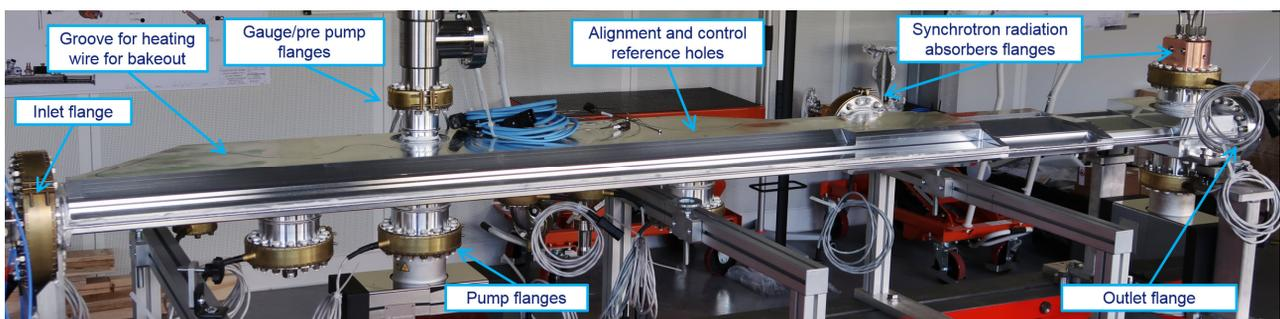
Figure 4: Series vacuum chamber (CH9) built by CECOM.
