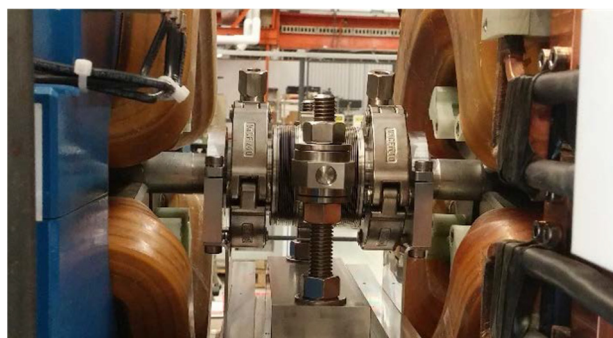
Figure 3: Narrow access between magnets to a compact BPM assembly demonstrated on a mockup.
