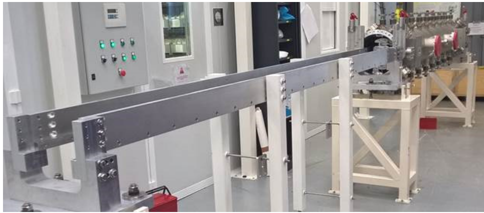
Figure 2: View of the tooling used to install the girders inside the vacuum chamber.
