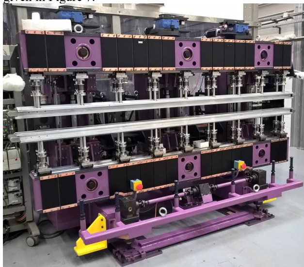
Figure 7: Jaw assembly reproducibility test.
