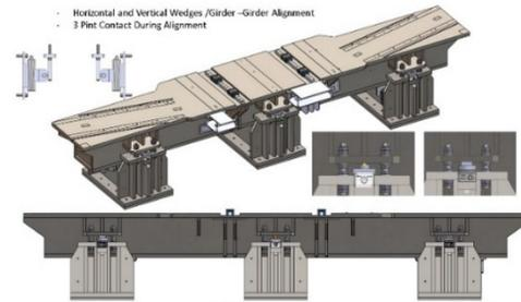
Figure 7: Girder adjusting system.
