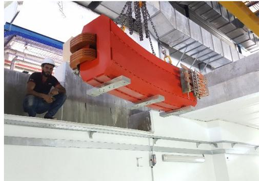
Figure 8: Dipole Bending Magnet.
