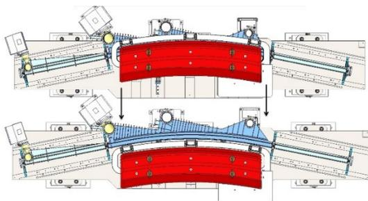
Figure 11: Pushing the dipole out.
