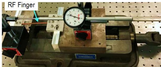
Figure 10: Test setup for cyclic fatigue testing of the RF fingers.
