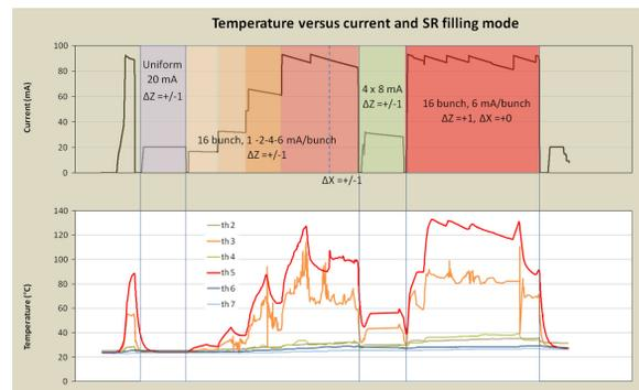
Figure 9: Temperature vs ring current and filling modes.
