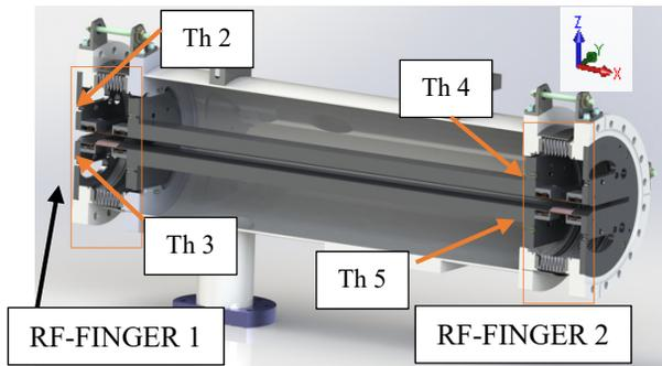
Figure 7: Cut view of the test chamber.
