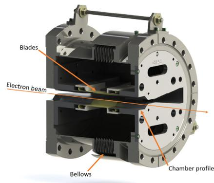
Figure 1: RF Finger placed in a bellows.
