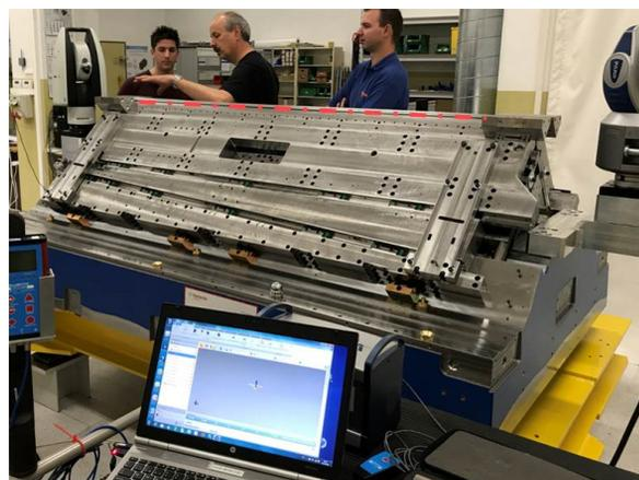
Figure 17: Measurement with laser tracker.
