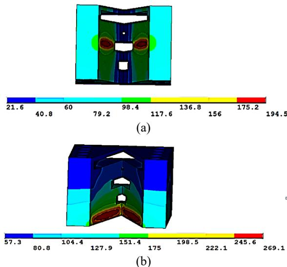
Figure 7: Temperature contours for slit design 2, (a) beam at the center of an aperture, (b) beam on a beam-stop position.
