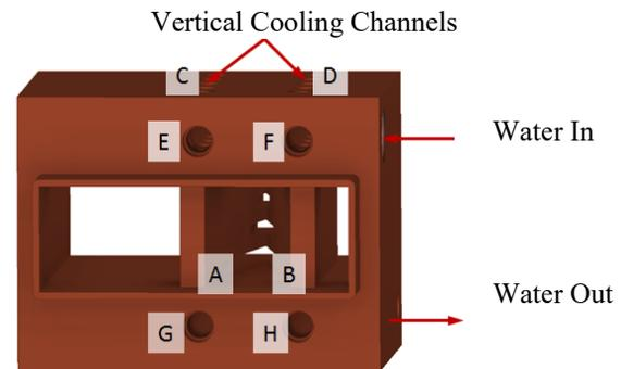
Figure 5: Slit design 2 with beam-intercepting inclined surfaces A and B. Vertical cooling channels C and D are interconnected by horizontal channel E, F, G and H.
