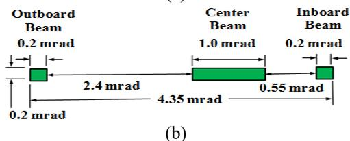
Figure 1: HEX wiggler x-ray source and beams, (a) power distribution of 4.3 Tesla SC wiggler, (b) 3 beams, fan sizes and spacings.
