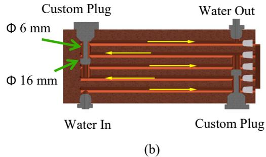
Figure 4: Cooling channels configuration, (a) C and D channels of  $\phi$  9.5 mm interconnected by channels E and F of  $\phi$  16 mm, (b) custom plugs for connecting the channels in series.
