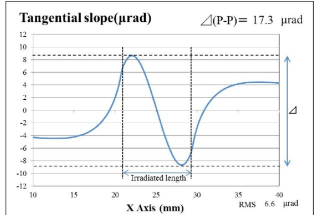
Figure 4: Tangential slope error of Si first crystal.
