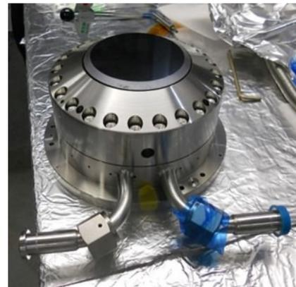
Figure 6: Si first crystal mounted to the manifold.
