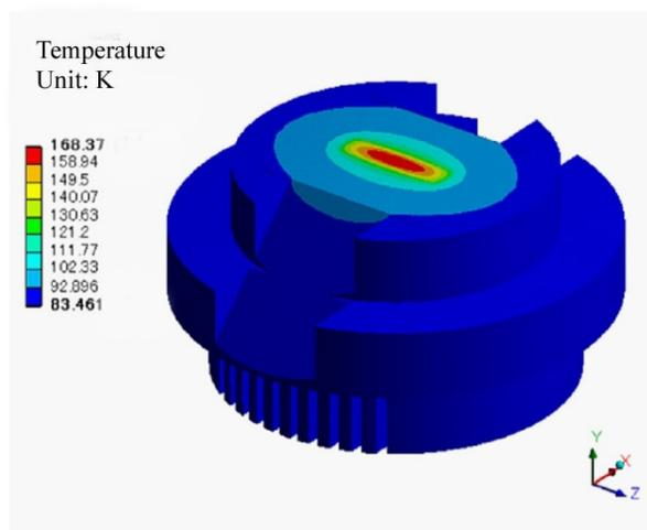
Figure 1: Temperature profile of the first crystal. Total heat load=2 kW; power density=7 W/mm<sup>2</sup>; foot print=33.6 mm x 8.51 mm (H x V); T-LN2=80 K; h=0.0103 W/mm<sup>2</sup>K. This calculation model is for the thermal design phase.
