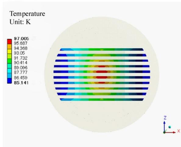
Figure 2: Temperature profile of the top of channel. The maximum heat flux of the channel is 0.18 W/mm<sup>2</sup>.
