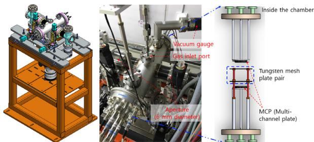
Figure 3: GMD installed at UH and schematic drawing.
