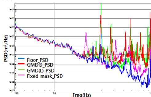
Figure 5: The characteristics of vibration displacement around GMD.
