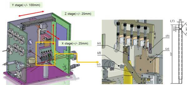
Figure 9: Sample injector: (a) pinhole position, (b) cross wire holder, (c) PD manipulator, (d) oxygen & humidity sensors (e), (f) sample catcher.
