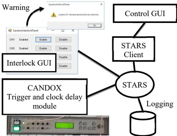
Figure 3: Software interlock system.
