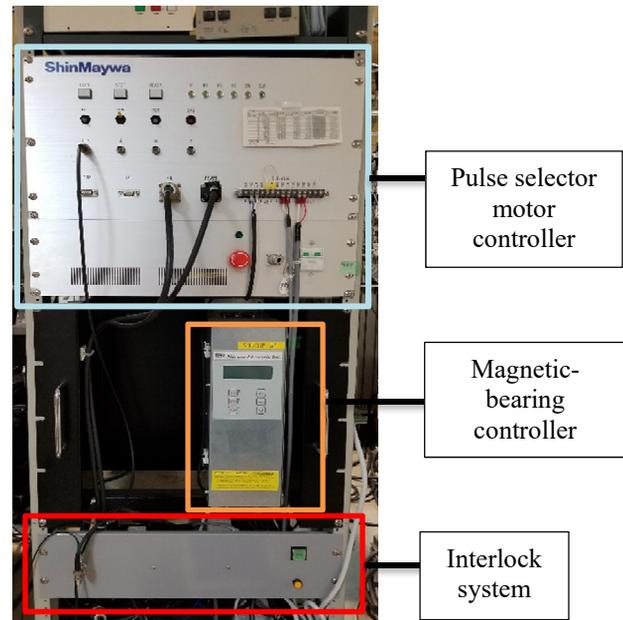
Figure 6: Interlock system and controllers.
