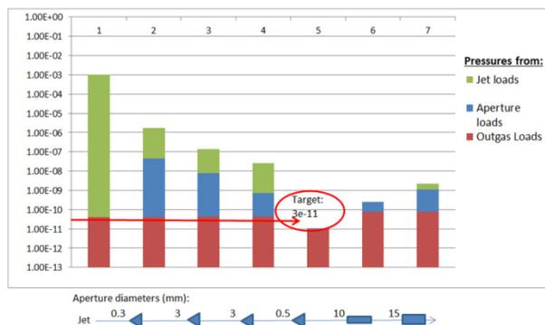
Figure 5: Calculated pressure profile in DREAM starting from the gas jet chamber on the left through 4 skimmers to the catcher chambers on the right. Starting with a pressure of  $1 \times 10^{-3}$  Torr in the gas jet chamber, the main chamber at bar graph position 5 should still be able to reach a base pressure of  $3 \times 10^{-11}$  Torr, but will be highly dependent on the outgassing rate of parts in the main chamber.
