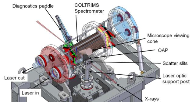
Figure 2: The DREAM interaction region noting positions of spectrometer, microscope view, diagnostics paddle, x-ray path, laser path, and optics support post with integrated scatter slits.
