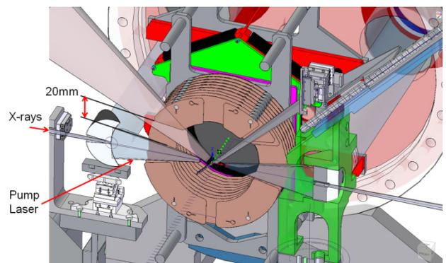
Figure 3: Cross section view at the center of the DREAM instrument. Note that the clearance cuts in the spectrometer voltage plates allow for 20 mm of vertical movement of the main chamber while the laser in-coupling and out-
