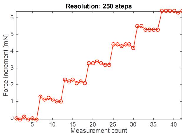
Figure 3. Resolution test results of the corrector.
