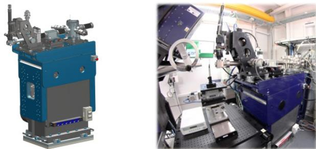
Figure 1: General overview of the Beam Conditioning Optics.
