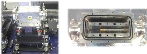
Figure 2: Images of the micro focusing lenses unit.
