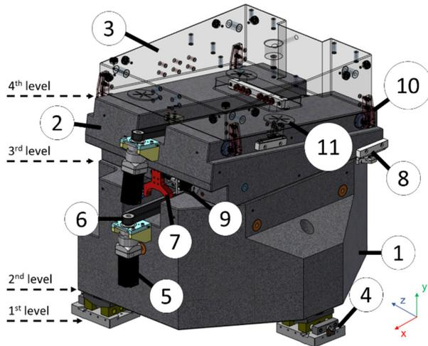
Figure 2: Three-part granite bench for the mirrors systems: (1) bottom granite; (2) middle granite; (3) top granite (transparent for visibility); (4) wedge-leveller; (5) stepper motor for  $T_x$ ; (6) timing belt for  $T_x$ ; (7) commercial air-bearing guiding for  $T_x$ ; (8) optical encoder; (9) power screw mechanism for  $R_y$ ; (10) commercial air-bearing for wedge; and (11) machined air-bearing pad.
