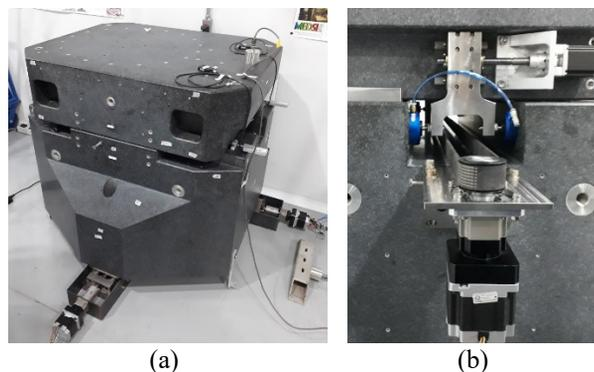
Figure 3: (a) 4CM granite bench assembled at the hall of the metrology building of LNLS; (b) Detail of  $T_x$  and  $R_y$  stepper-driven actuation mechanisms with the timing belt and power screw, guided by the commercial air pad.
