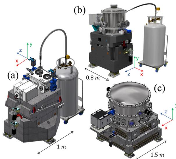
Figure 1: Optical systems mounted on granite benches: (a) mirror; (b) double channel-cut monochromator (4CM); and (c) High-Dynamic Double Crystal Monochromator (HD-DCM) (Beam direction: +z. Vertical up: +y).
