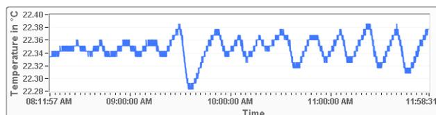
Figure 4: Plot showing typical stability of temperature in the environmental enclosure over a period of 4 hours.
